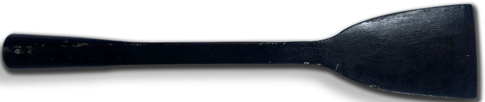
The cutting spade, or “espeiro” how it was called by whalers, was a tool used to butcher sperm whales. It consisted of a cutting blade and a long wood cable, whose usefulness was known in the butchering platform, where the different animal body tissues were taken apart in order to maximize the processing and extraction of these animal's products.
